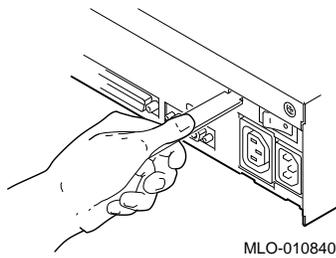
4. Pivot the cover on the tabs that run along the system unit's front edge.
