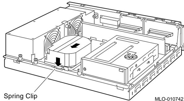
3. Lift the disk drive up from the drive mounting shelf and release the spring clip.
