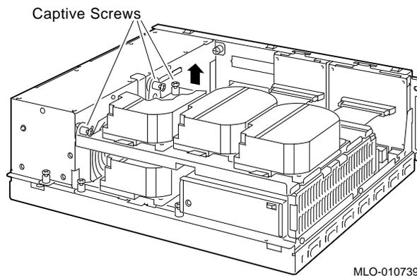
3. Lift the left side of the shelf and pull the shelf to the left until the tabs on the right clear the cutouts in the lower drive shelf.
