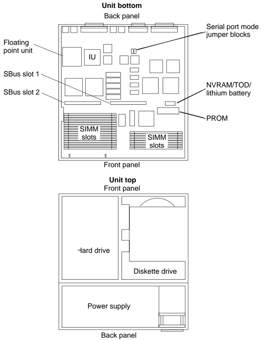
Figure 3-2 Top View of System Unit and Subassemblies
