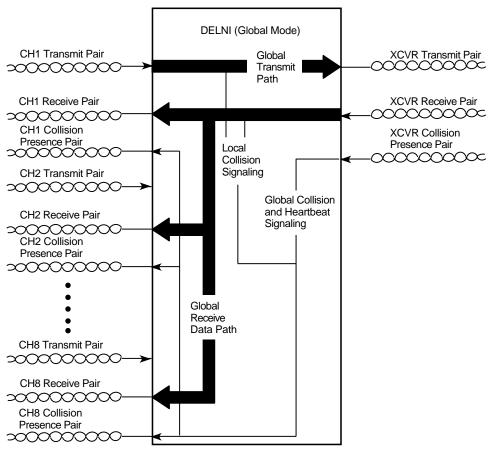
Figure 3–3 GLOBAL Mode Signal Flow Diagram
