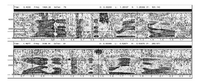
**Figure 2**Two Spectrograms of the Utterance "Line up at the screen door." The upper spectrogram is the author's speech. The lower spectrogram is synthetic speech produced by DECtalk Software.
