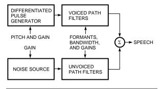
**Figure 6**Basic Architecture of the Vocal Tract Model
