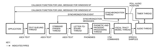
**Figure 3**The DECtalk Software Architecture for Windows NT
