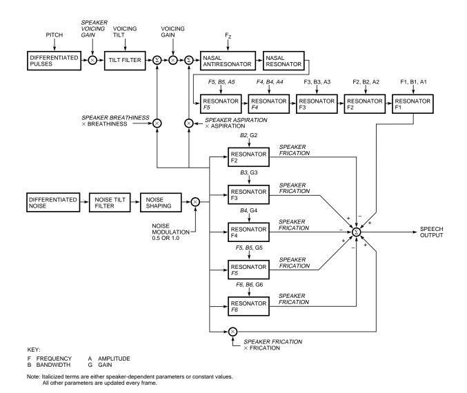
**Figure 7**The DECtalk Software Vocal Tract Model (also known as the Klatt Synthesizer)
