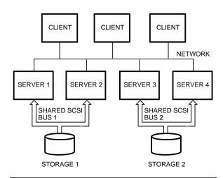
Figure 2 Asymmetric Configuration of ASE
