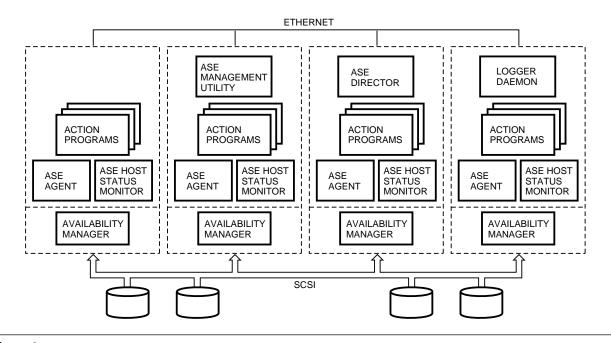
Figure 4 ASE Component Configuration
