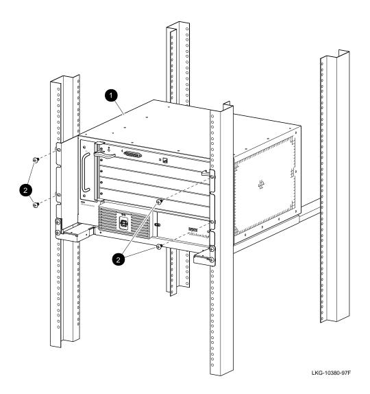
Figure 10-1 Detaching the System from the Rack
