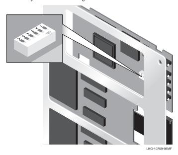
When the module is installed into the chassis the lettering on the switch pack is upside down (switch 6 being the left most).
