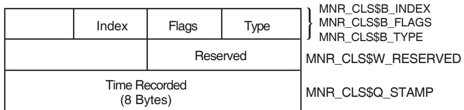
Figure A-6 Class Header Format - Alpha and Integrity servers
