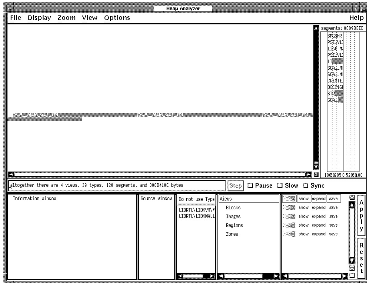
Figure 12–12 Incrementing Memory Allocation Indicates a Memory Leak
