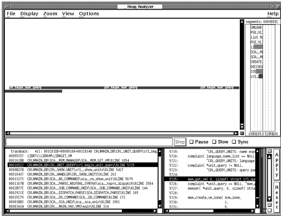
Figure 12–14 The Click on Traceback Entry Shows Associated Source Code
