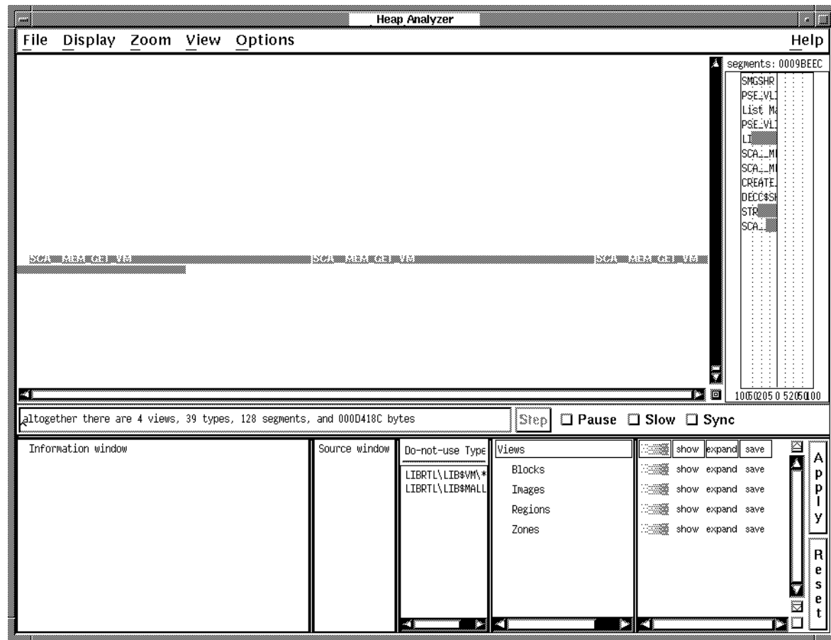
Figure 12–12 Incrementing Memory Allocation Indicates a Memory Leak
