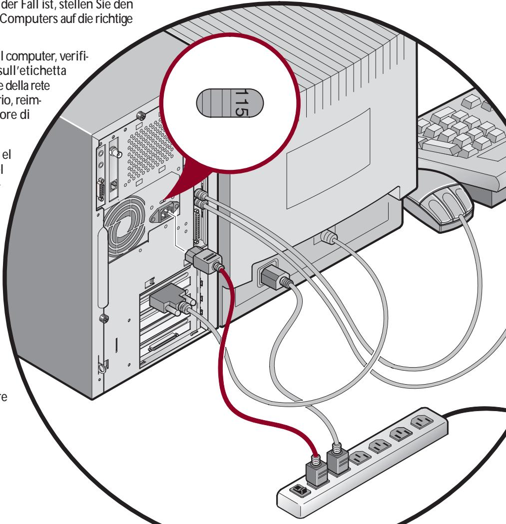
**English** If your computer came with integrated network capability, you have connectors for 10Base-2 (Ethernet ThinWire) and/or 10Base-T (Twisted Pair) network cabling. Contact your network administrator before connecting to a network.
