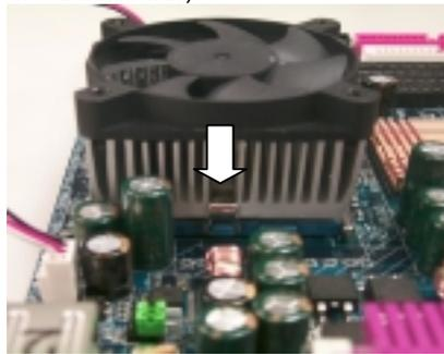
5. Hook one end of the cooler bracket to the CPU socket.
